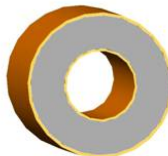
12. The space between PVC pipes Ø 50 and Ø 100 is filled with Simprolit monolith
